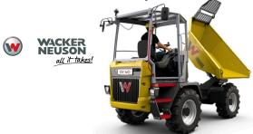
Offering an enhanced degree of safety and productivity on the job site. The DV60 has a dual view, allowing the operator to always have full visibility: when unloading, the driver looks in the direction of the skip, before continuing driving, the operator swivels the seat and console so they are facing in the driving direction.
